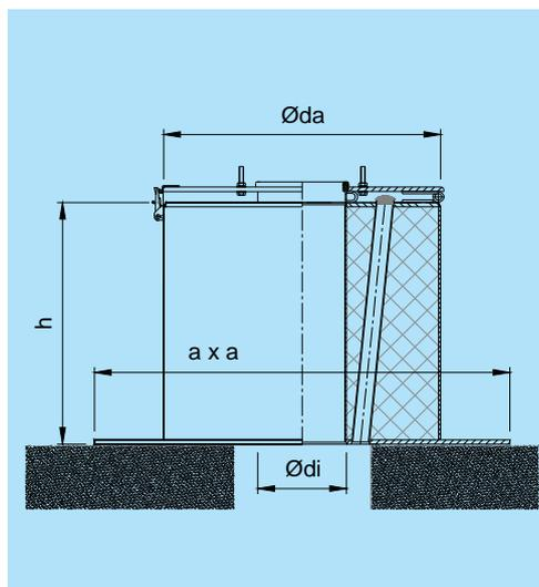
The sound-absorbing upstand is used for damping the sound power radiated into the suction line.
