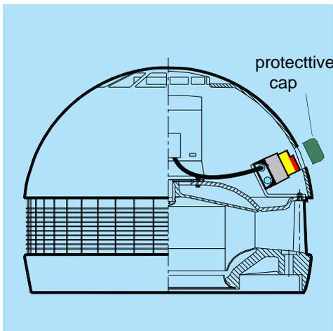
The repair switch RS is used to disconnect the fan completely from the mains in cases of repair and maintenance. This excludes the risk of accidents arising from unauthorized activation.
